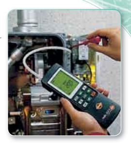
The Testo 312-2 measures low pressure from 40/200 mbar compared to the Testo 312-3 model which measures high pressure from 300/6,000 mbar (DVGW approval according to TRGI).
