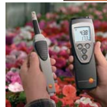
Probe head on radio handle (optional) for wireless data transmission over large distances
