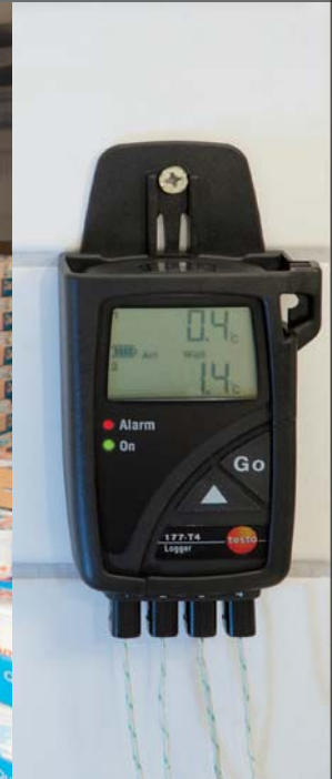
Simultaneous temperature measurement at up to 4 different sites
