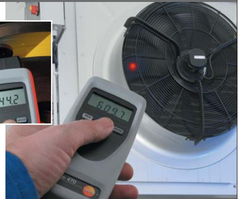
testo 465 and testo 470, non-contact (optical) rpm measurement on rotating parts
