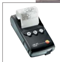
Cyclic printing of readings on the Testo fast printer, e.g. once per minute (with testo 635-1)
