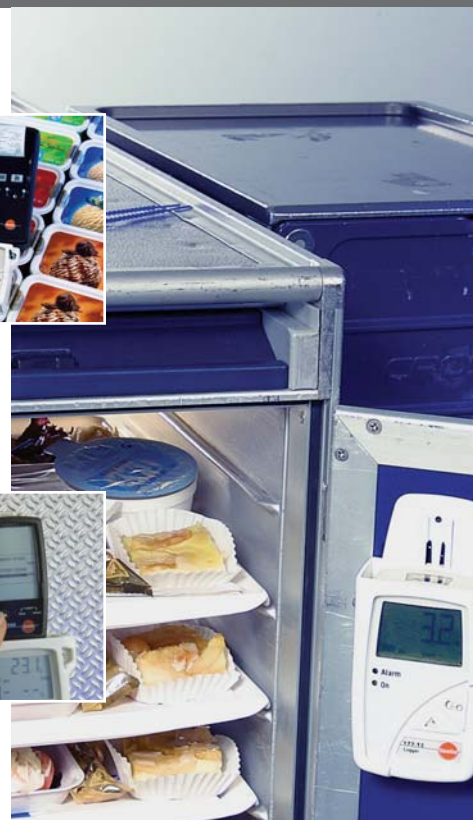
Long-term temperature logging with immediate display of limits exceeded e.g. during transport, in refrigerated rooms, warehouses etc.
