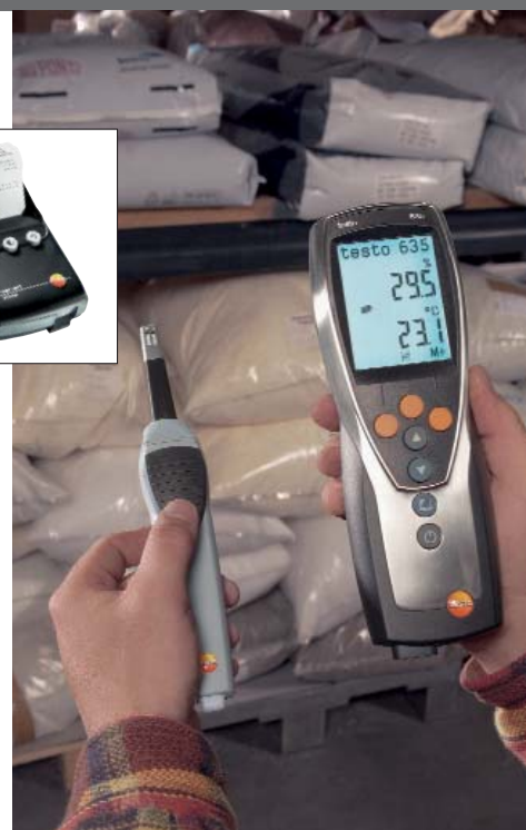
Wireless measurement of warehouse temperature and humidity, with radio handle and attachable humidity probe head
