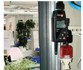
Read out the data stored in the logger via the PC network using the Ethernet adapter
