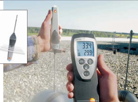
Monitoring temperature at exhaust outlets
