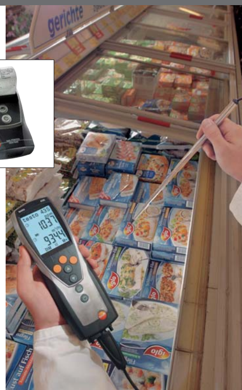
Monitoring air turnover in a refrigeration chest
