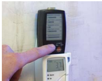
The testo 580 data collects data on site for upload to PC and analysis
