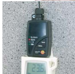
testo 581 alarm signal output for reliable warning of limits exceeded
