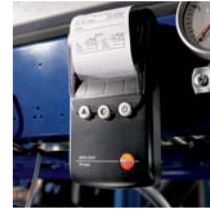
On-site printout of measurement data on infrared printer
