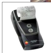
Fast documentation through measurement data printout on location
