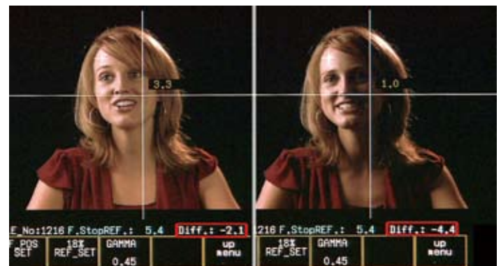
CINELITE can be a useful lighting tool by helping you measure f-stop values in real time.
