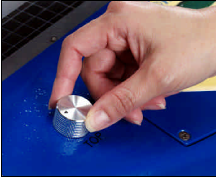
Figure 4: Lighting Intensity Control
