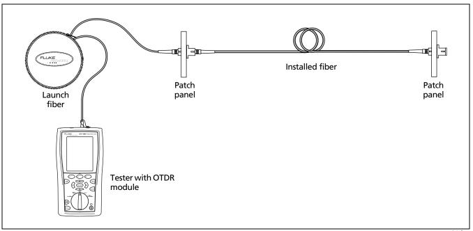
Figure 5. Connecting the OTDR to Installed Fiber (no receive fiber)
