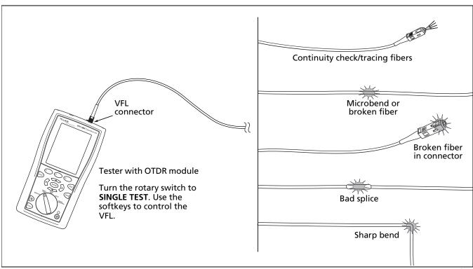
Figure 12. Using the Visual Fault Locator
