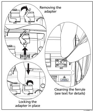
Figure 13. Cleaning the OTDR Ports
