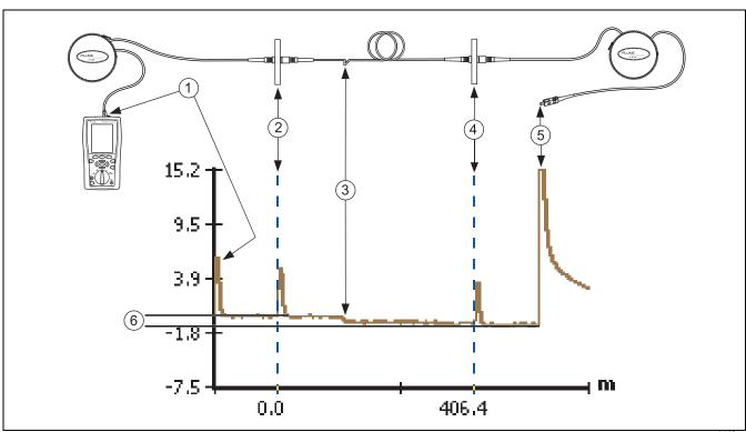
**Figure 10. Typical OTDR Trace Features**
