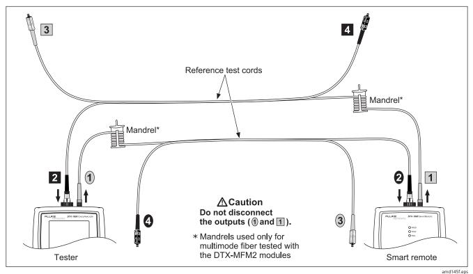
Figure 8. Smart Remote Mode Reference Connections (Method B)
