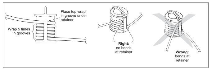
Figure 5. Wrapping a Reference Test Cord Around a Mandrel
