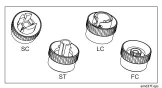
Figure 3. SC, ST, LC, and FC Connector Adapters
