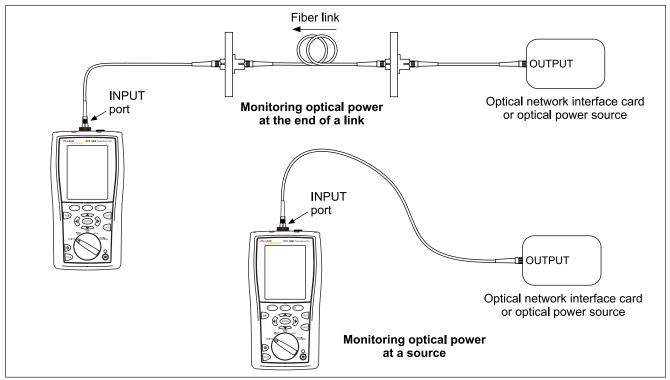
Figure 19. Connections for Monitoring Optical Power
