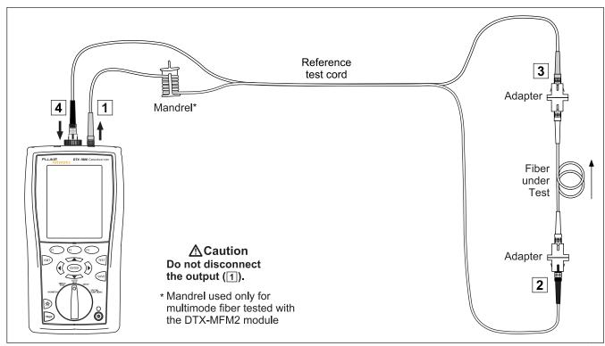
Figure 12. Loopback Mode Test Connections (Method B)
