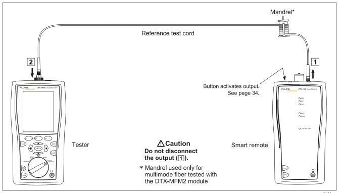
Figure 14. Far End Source Mode Reference Connections (Method B)
