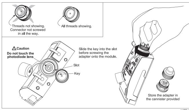
Figure 4. Installing the Connector Adapter
