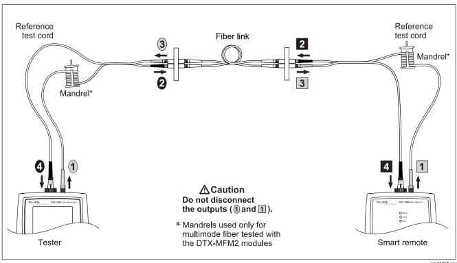
Figure 9. Smart Remote Mode Test Connections (Method B)
