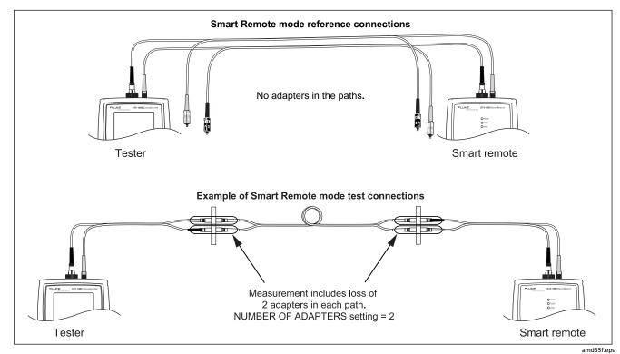
Figure 6. Example of How to Determine the Number of Adapters Setting (singlemode example; mandrels not used)
