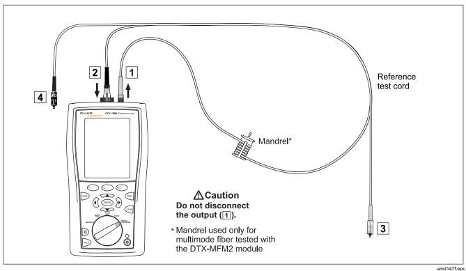
Figure 11. Loopback Mode Reference Connections (Method B)
