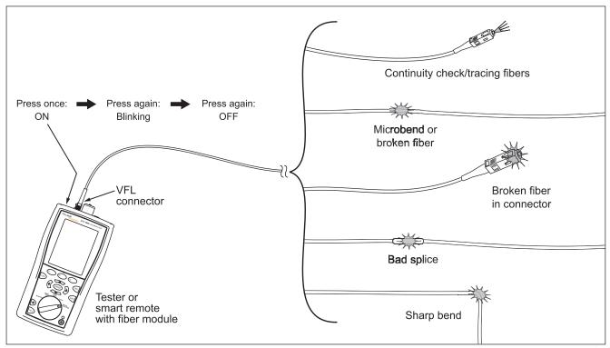
Figure 17. Using the Visual Fault Locator
