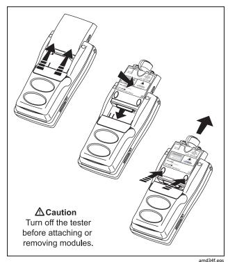
Figure 1. Installing and Removing Fiber Modules
