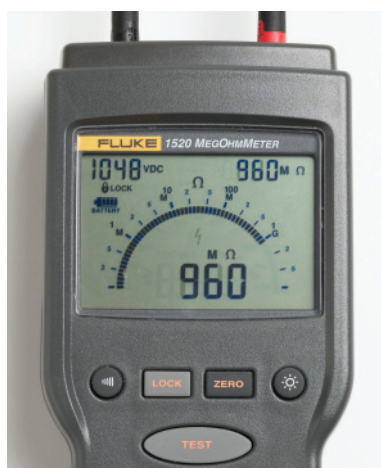
At 960 MΩ, this cable tests satisfactorily.
