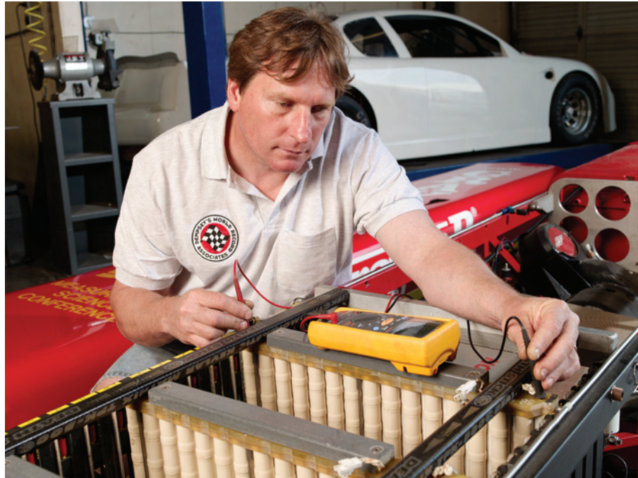
Racing team manager Gus Fowlie taking a DC voltage measurement across one of the battery packs in White Lightning that hold multiple C size Nickel-Metal Hydride batteries.
