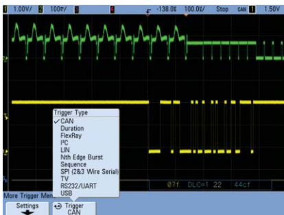
Trigger on and decode CAN serial packets.
