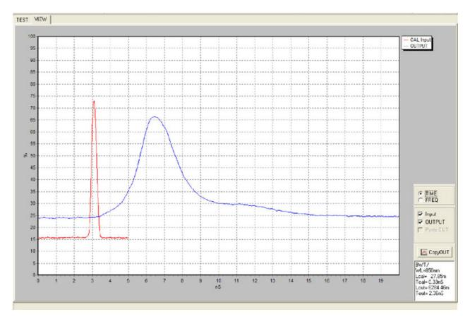
Here are pulses from a sample test of 3.5 km of fiber viewed in the "time domain" like an oscilloscope. The red pulse is the test pulse from the 850 nm laser transmitter. Note it is only about 0.3 ns wide (FWHM – full width half max). After traveling down the fiber, you can see the pulse broadening, just like an electrical pulse is broadened by a filter.
