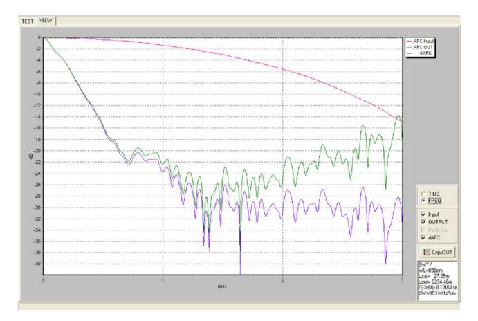
Here is the same data after analysis. We are looking at the frequency domain now, where we see the attenuation of the fiber in dB on the Y-axis and the frequency on the X-axis. The red line is the input and the green line the output. The blue line shows the difference between the two which is the affect of the bandwidth of the fiber itself. From the data panel on the lower right, we see the calculated bandwidth of the fiber is 536 MHz-km.
