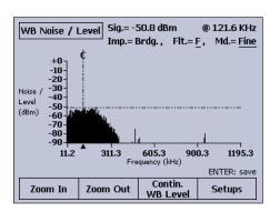
Interference from other services in a binder group, such as HDSL in this example, are easily detected using the CopperPro's wide band noise/level spectrum measurement. Interference masks simplify identification of the source.
