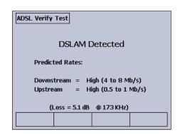
Using special software emulation, the CopperPro activates communications with the central office DSLAM and measures performance on the line.
