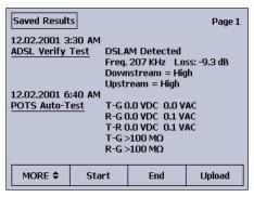
Test results are automatically saved for printing or uploading to PC.
