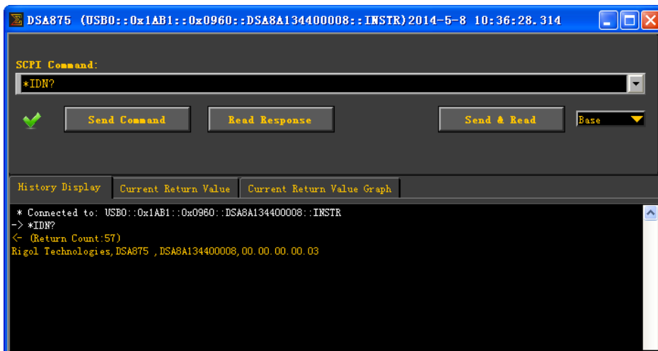
Figure 3-2 Write and Read Commands via USB
