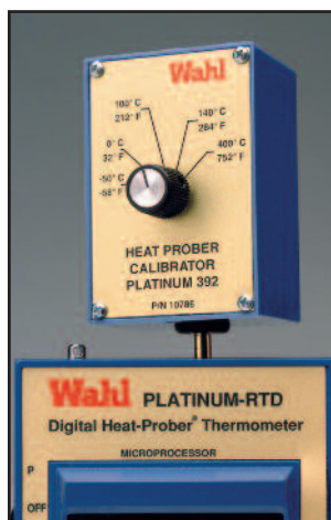
Platinum RTD Meter 392AMF shown with 5-point calibrator CAL392-HT
